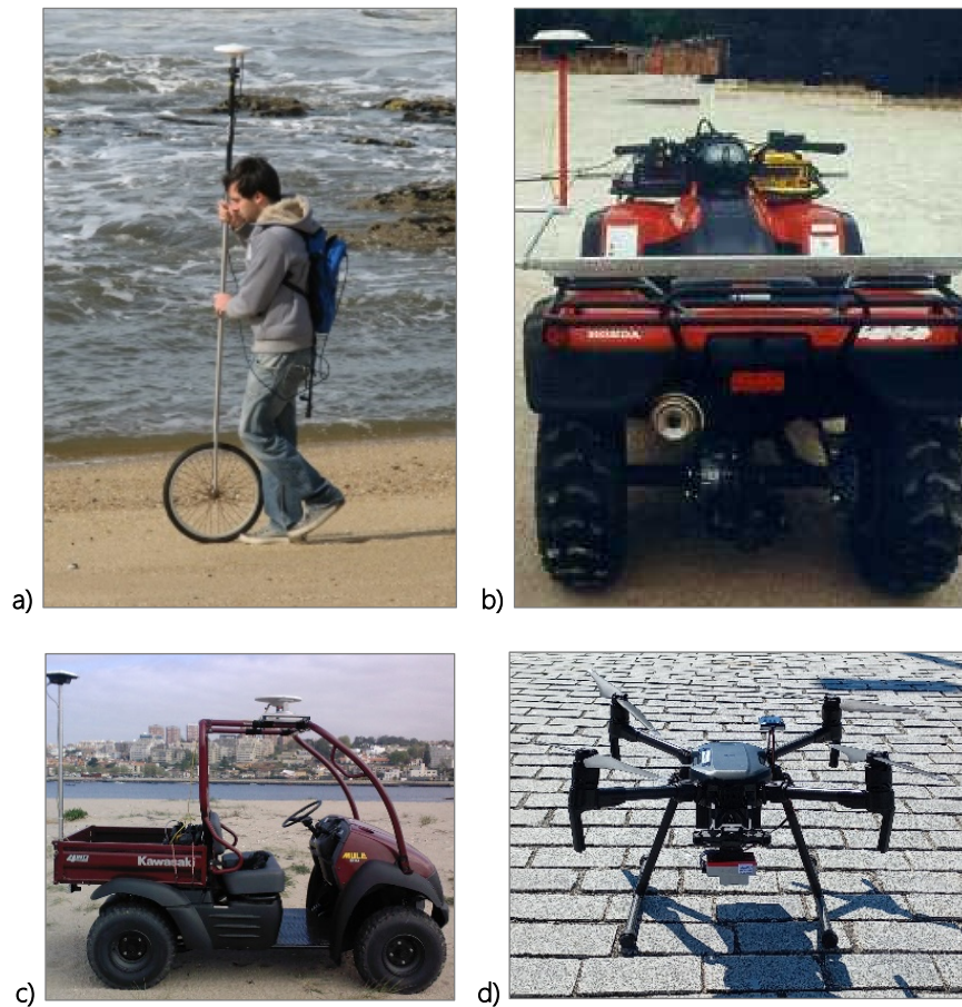
Figure 2: Survey methods: walking wheel (a), moto quad (b), utility vehicle (c) and UAS (d).
