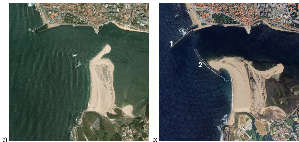
Figure 1: The Douro sand spit in June 2006, i.e. before the intervention (a) and in July 2023, with the cities Porto on the upper, northern margin and Vila Nova de Gaia on the lower, southern margin; 1: extended northern breakwater, 2: detached breakwater (Images: GoogleEarth, Maxar and Airbus).
