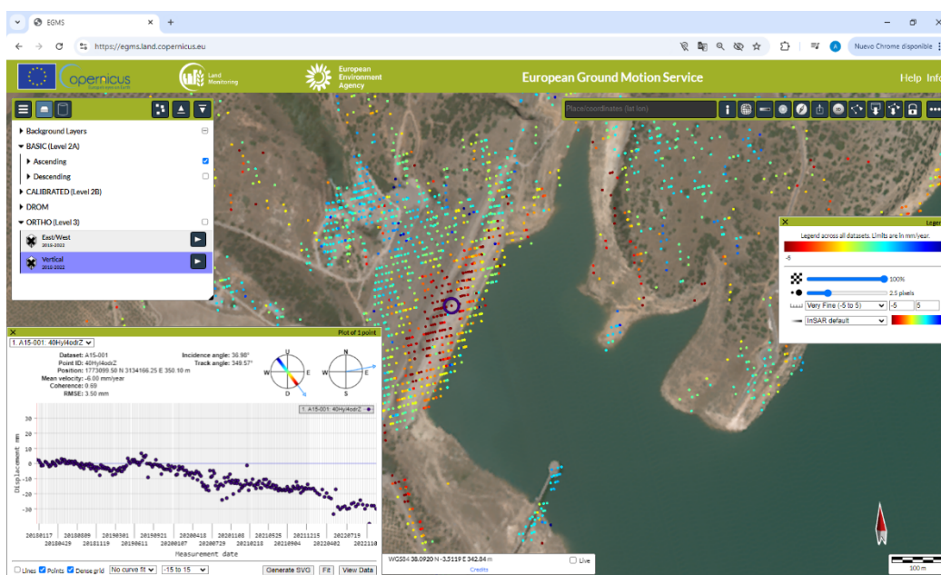
Figure 3: Map of the average LOS velocity using ascending Sentinel-1 imagery processing for 2018–2022 over the Giribaile Dam (EGMS).
